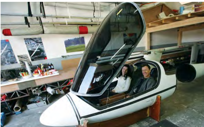
Eric Raymond and his fiancée Irena try out the cockpit of the Sunseeker III. Irena is a glider pilot and president of the Slovenian womens pilots association. The aircraft controls are installed. The seats will be made with comfort in mind for long flights and will recline so one pilot can rest while the other flies.
