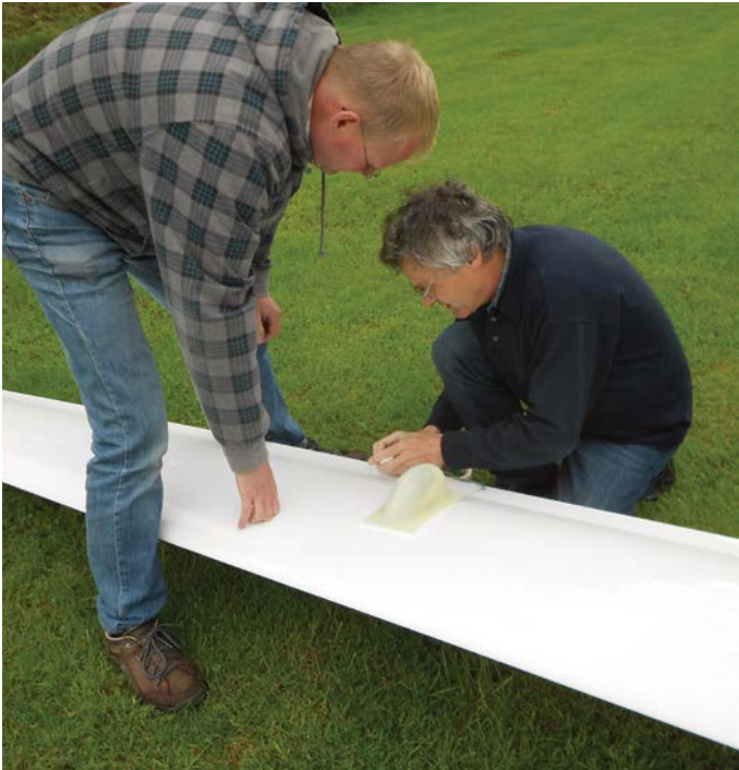
L: Designer Martin Hider and Schleicher's General Manager Uli Kremmer fitting a device for flutter testing as part of the final certification process. Top R: Terry preparing to fly the ASH 30 Mi. Middle and bottom R: The Schleicher factory. Below: AHS 30 Mi
