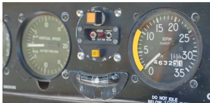
The little yellow button with CHT on it flashes to show the pilot when the max cylinder head temperature is exceeded.
