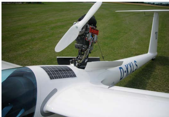
A SOLO-2350 engine, solar panel, and bug wiper "garage" are all features of the LS-10. The bug wipers retract into a recess in the fuse so they sit flush. If the optional bug wipers are not installed when you buy an LS10 or DG 808cc there is a little cover the same shape stuck over the recess. DG is the only manufacturer that supplies this as an option.
