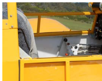
The door hinge, showing the gusset in the corner
