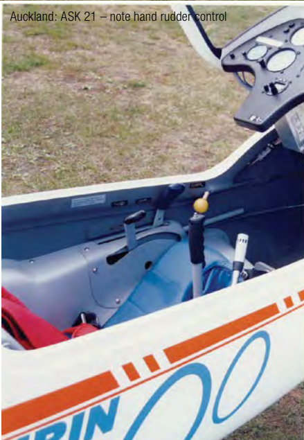
Auckland: ASK 21 – note hand rudder control
