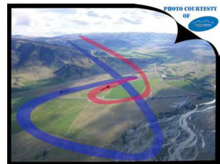
Take off runway 09 in light winds with blue showing the climb and red showing the descent and return to runway 27.
