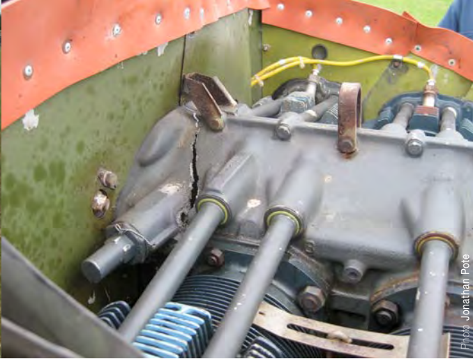
A: what little oil remained to leak out after DML came to rest. B: The split crankcase. You could see right through the engine.
