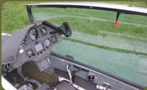
Instrument panel - the hinged instrument panel makes for easy access and has plenty of room for instruments
