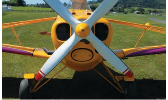
The heavy metal disc can be seen behind the prop.
