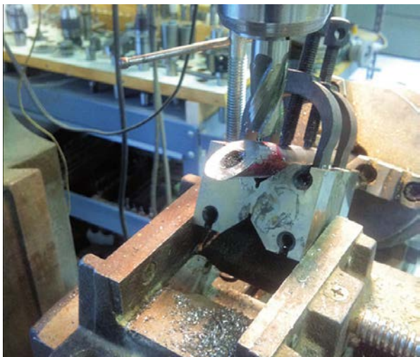
Pins connecting inner and middle wing panels are shaped to contours of wing.
