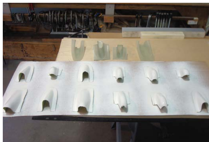
Flap and aileron fairing moulds built, fabricated and painted.
