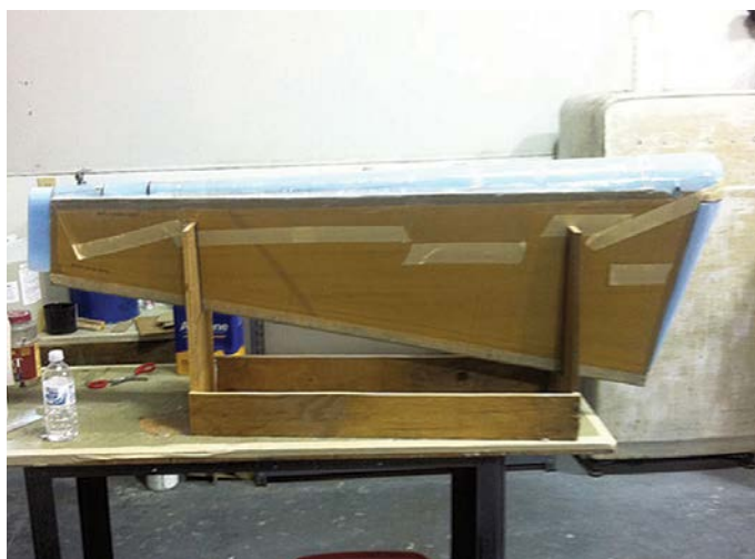
I-R Nose of rudder and tips being fabricated, fitting rudder to vertical stabilizer, templates are used to form tracks on middle wing.
