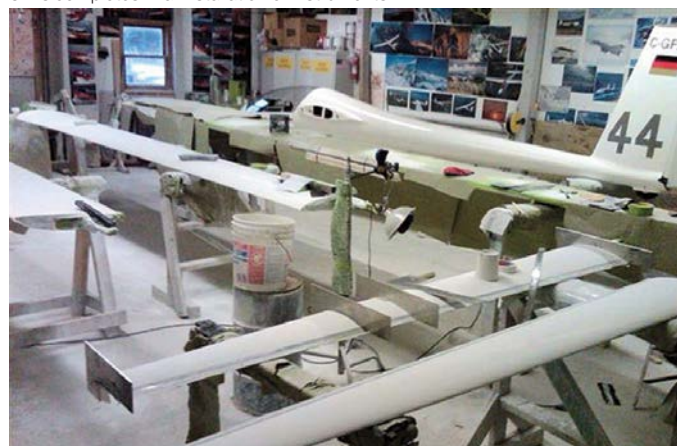
Contouring leading edge of outer panels using templates.
