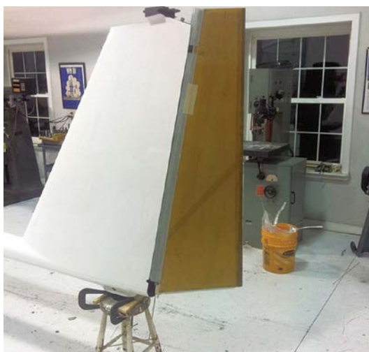
I-R Nose of rudder and tips being fabricated, fitting rudder to vertical stabilizer, templates are used to form tracks on middle wing.
