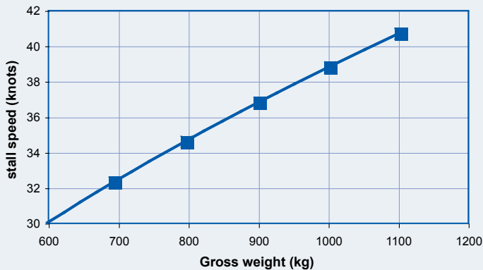
GRAPH 3 Effect of load on stalling speed of a Piper Cub
